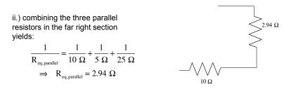
iii.) finally, combining that parallel equivalent resistance with the series 10 ohm resistor yields an overall equivalent resistance of:
